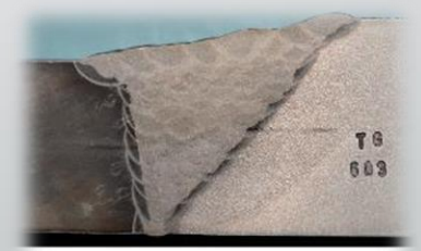
Weld Procedure / Welder Qualification WPQR 603 Welder: Tim Graham
